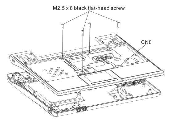
Figure 4-11 Removing the top cover
